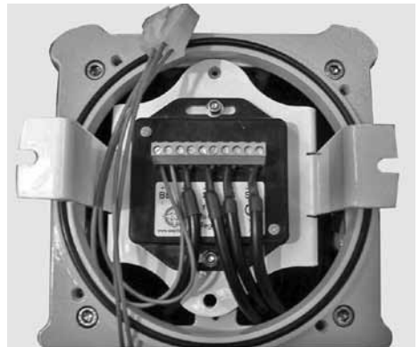
SL10 AMP Regulator shown when correctly fitted
