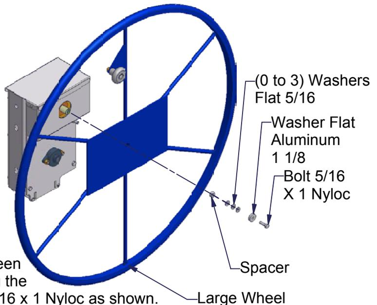
NOTE: You should be able to slide a piece of paper in the gap between sticker in the center of the wheel and the washer. The wheel should turn 1/8 to 1/4 turn prior to engaging the Washer Flat Aluminum 1 1/8.
