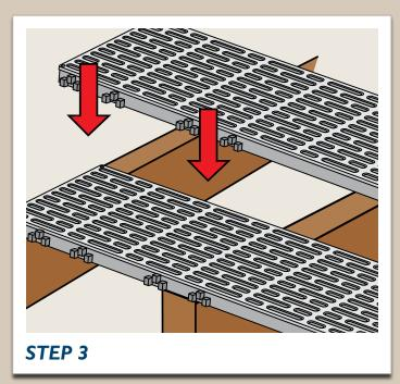
Using the interlocking system, lay the next ThruFlow $^{\text{\tiny M}}$  panel and repeat the fastening process.
