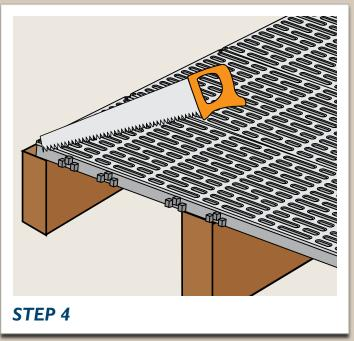
To finish the installation, remove the last row of interlocking tabs, using any traditional hand or electric saw.
