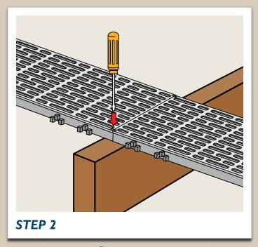
Lay the first  $\mathsf{ThruFlow}^\mathsf{T}$  on the substructure and fasten using a pan head screw. Hand tighten each screw.
