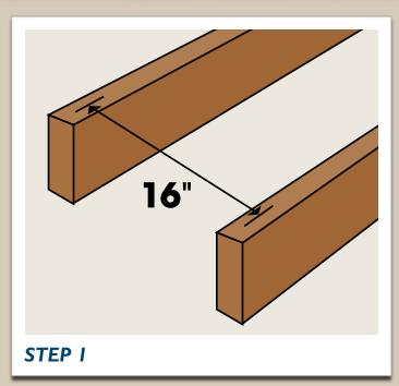
Substructure to be constructed with cross-members equally spaced on 18" centres (3' planks), 16" centres (4' planks) and 15" centres (5' planks).
