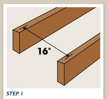
Substructure to be constructed with cross-members equally spaced on 18" centres (3' planks), 16" centres (4' planks) and 15" centres (5' planks).
