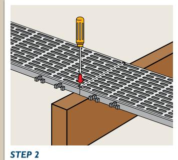
Lay the first ThruFlow<sup>m</sup> on the substructure and fasten using a pan head screw. Hand tighten each screw.
