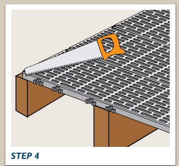
To finish the installation, remove the last row of interlocking tabs, using any traditional hand or electric saw.
