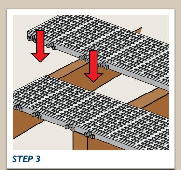
Using the interlocking system, lay the next ThruFlow<sup>T</sup> panel and repeat the fastening process.
